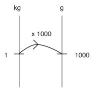
The diagram shows that 1 kilogram and 1000 grams are the same because they are at the same level on the scale and that you have to multiply by 1000 to convert 1 kg to grams. The same relationship clearly holds for other amounts
